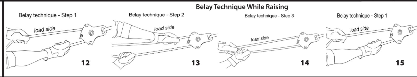
Note: it is an advantage to use a "static" kernmantle rescue belay rope with 'low' stretch properties.
